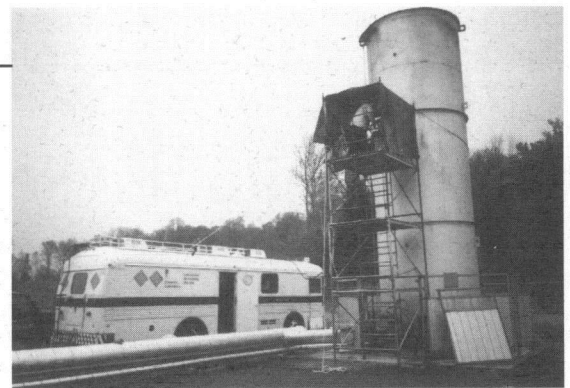
All in a day's work: taking emission samples from a stack at a landfill near Ottawa. Photo courtesy of Source Measurement Section, PMD.
