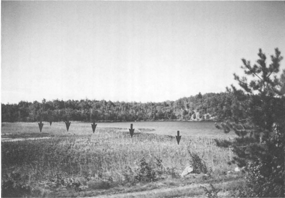
PLATE 1a OVERVIEW OF T-4 CATTAIL STAND (OLIVE). The shallow tailings beach was submerged by the end of August, 1982. The dried plants are growth from 1981 at the border of the dry portion of the tailings. Arrows indicate six permanent quadrats distributed throughout the stand.
