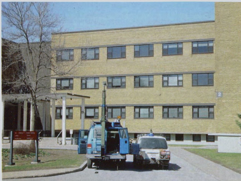
Transmit vehicle and broad face of the building section where the measurements were made, showing the antenna mast elevated from the rear of the vehicle housing the transmitter.
