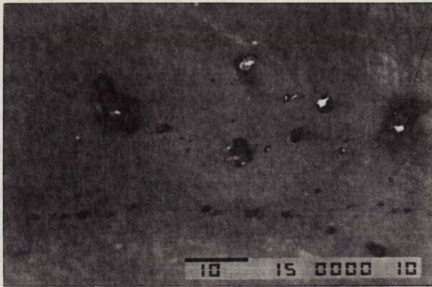
FIG. 27 SEM (NORMAL) PHOTOGRAPH OF EXPOSED KAPTON SAMPLE (1500 X)
