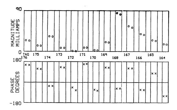
Figure 10 The RF currents flowing on the towers of the "north" power line of Figure 4.
