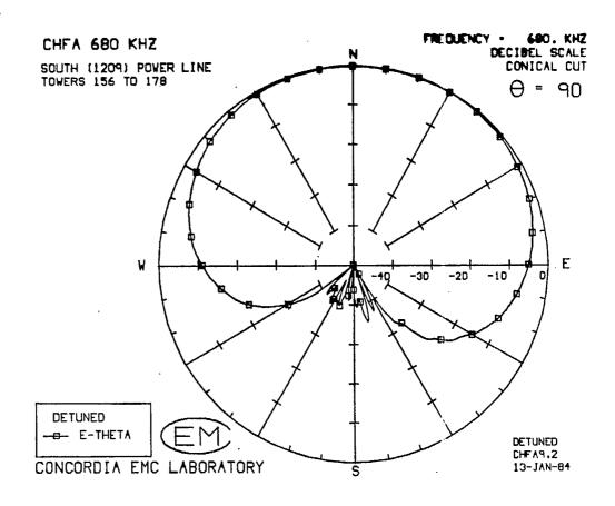
Figure 15(a) Azimuth pattern of CHFA near the "southeast" power line, which has been "detuned" by isolating towers number 176, 175, 173, and 172 from the skywire.
