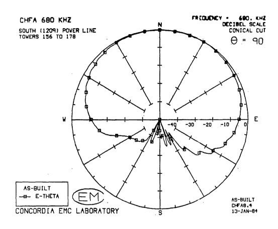
Figure 8(a) Computed azimuth pattern for CHFA radiating in the presence of the segment of the "southeast" power line of Figure 5.
