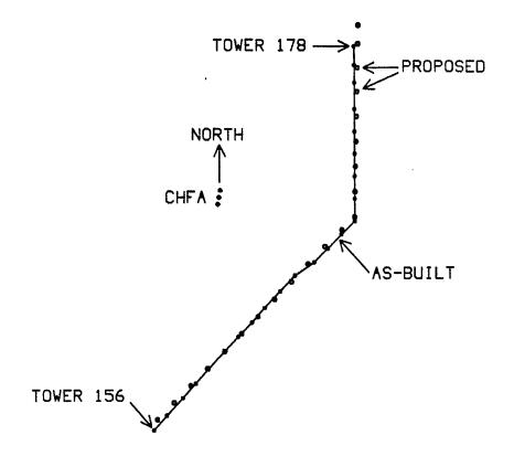
Figure 5 The computer model of the "southeast" power line used in the present study includes as-built towers 156 to 178, and is compared in this figure with the tower locations of the proposed power line, used in Reference (1).
