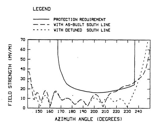
$\frac{\text{Figure 15(b)}}{\text{protection requirement.}} \quad \text{The "detuned" pattern meets the protection requirement.}$
