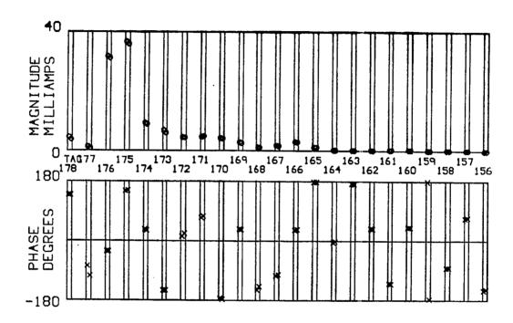
Figure 11 The RF currents flowing on the towers of the "southeast" power line of Figure 5.
