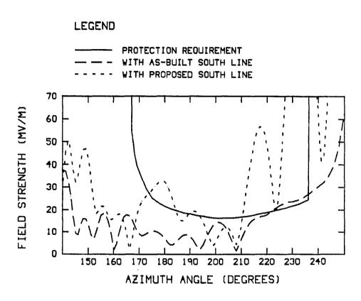
Figure 9(b) The "proposed" and "as-built" patterns are compared in the minimum.
