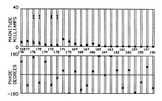
Figure 16 The RF currents flowing on the towers of the "detuned" southeast line. Towers marked with an "I" are isolated from the skywire.
