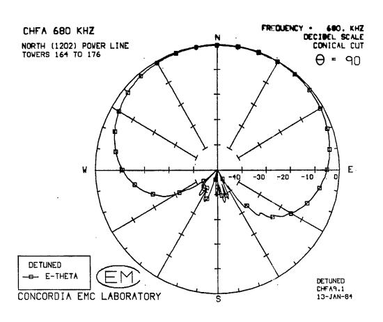
Figure 13(a) Azimuth pattern of CHFA near the "north" power line, which has been "detuned" by isolating towers number 174, 168, 167, and 165.
