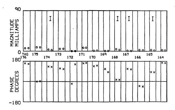
Figure 14 The RF currents flowing on the towers of the "detuned" north line. Towers marked with an "I" are isolated from the skywire.
