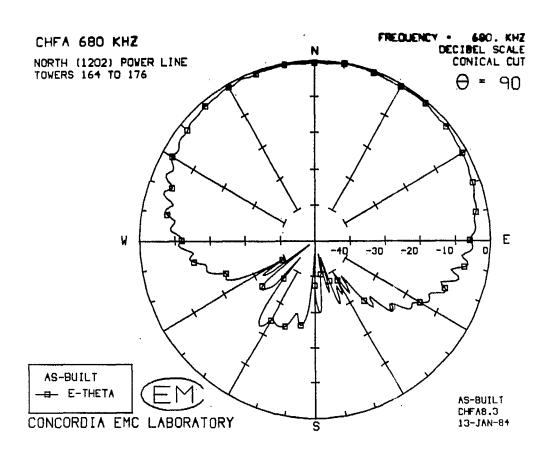
Figure 6(a) Computed azimuth pattern for CHFA radiating in the presence of the segment of the "north" power line of Figure 4.
