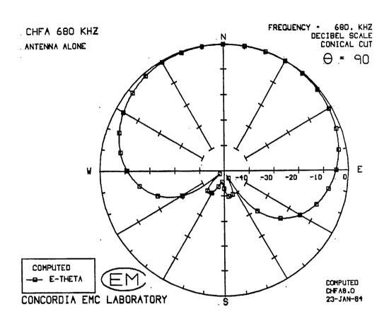
Figure 1(a) The computed azimuth pattern of station CHFA at 680 kHz. The station must maintain a stringent protection requirement from azimuth 167 to azimuth 236 degrees.
