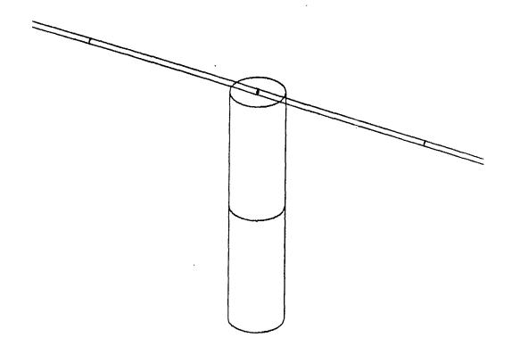
Figure 3 The model of the type Z7S tower of Reference (1) represents the tower with a wire 8 m in diameter, with a single overhead skywire 0.76 m in diameter.
