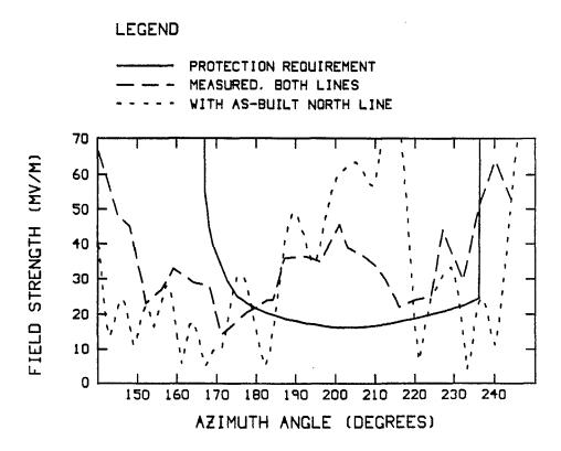
Figure 6(b) Comparison of the computed field strength for CHFA plus the "north" power line, with the CBC's measured field strength.
