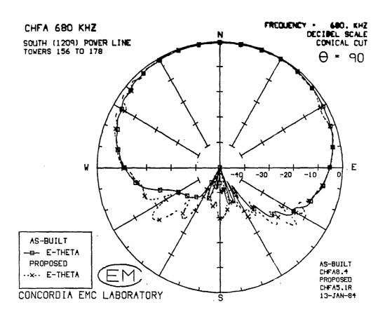
Figure 9(a) Comparison of the azimuth pattern of CHFA plus the as-built "southeast" power line with that of CHFA plus the proposed power line.
