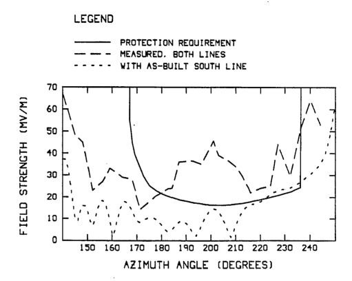
Figure 8(b) Comparison of the computed field strength for CHFA plus the "southeast" power line with the CBC's measured field strength.
