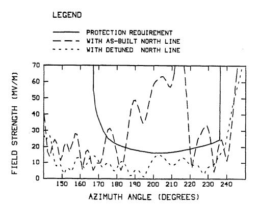
Figure 13(b) The "detuned" pattern meets the protection requirement.
