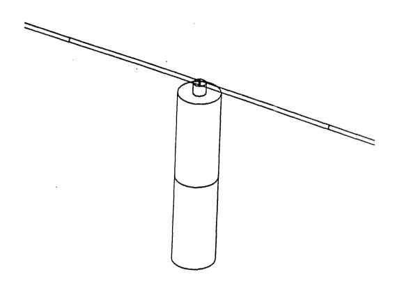
Figure 12 Modification to the model of Figure 3 to include a short segment at the top of the tower, which is "open circuited" with a large series resistor in order to "isolate" the tower from the power line.
