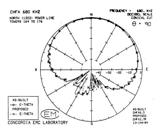
Figure 7(a) Comparison of the azimuth pattern of CHFA plus the as-built "north" power line with that of CHFA plus the proposed power line.
