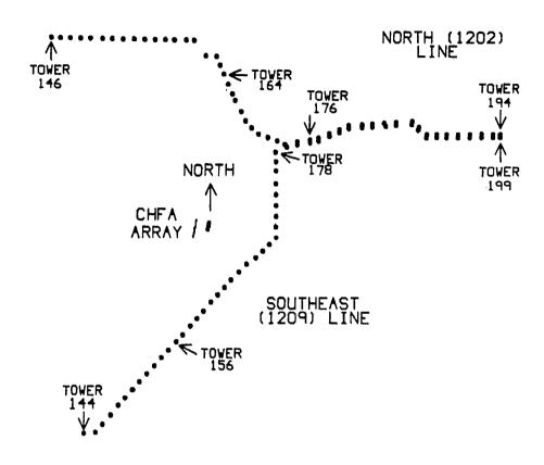
Figure 2 Plan view of the CHFA array and the two nearby high voltage power lines. The closest towers to CHFA on the north line are about 3.5 km away, and the closest towers on the southeast line are about 1.8 km distant.
