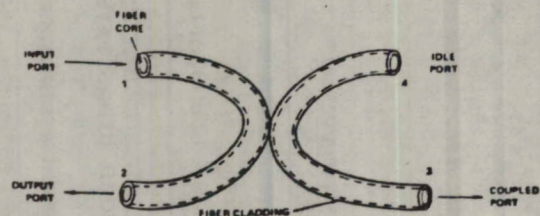
Fig.8.1b: Bringing Cores of Fibers Close Together 2
