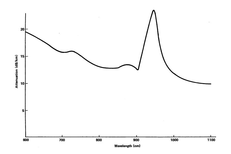
Figure 6.2 Fibre Attenuation v Wavelength. Based on Corguide Figures
