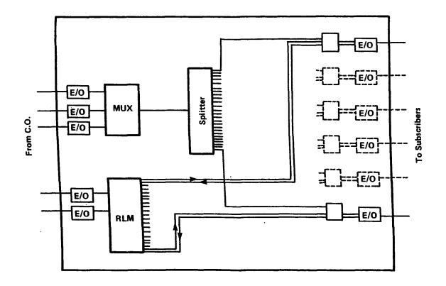
Figure 6.1 A Simplified Remote Switch Without Video Switching
