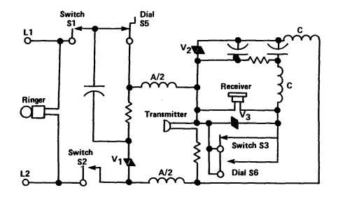
Figure 3.1 Schematic Diagram of 500D-Type Telephone Set
