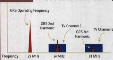
to the desired signals. If the harmonics fall on another locally used frequency, such as a television channel, they are likely to cause interference. The diagram at left shows how a signal from a GRS station may interfere with television reception.
