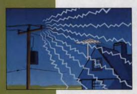
This type of disruption sounds like sizzling, sparking, intermittent or continuous crackling and appears and varies in intensity with weather conditions (dry or damp weather, wind). Additionally, if the result of the breaker test indicates that the source is outside the home, there is a good chance the interference is caused by faulty components in electrical power lines in the surrounding area.
