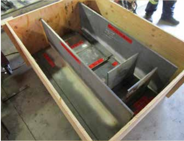
Figure 7. Material and weld samples from the future HMCS Protecteur .
