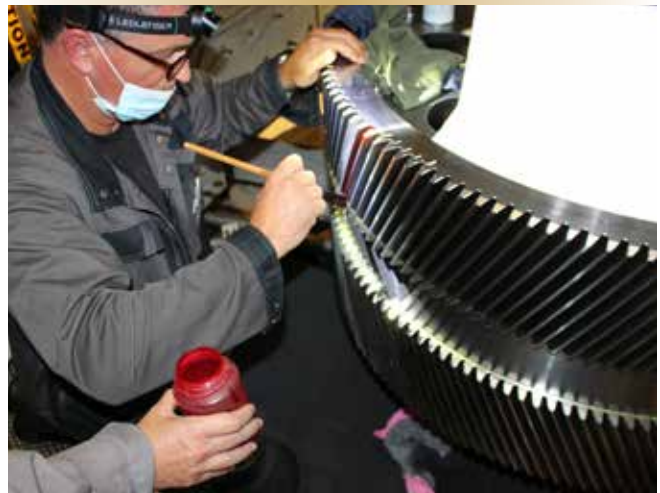
Figure 3. Painting sample teeth with Dykem Red for verifying correct gear meshing under at-sea operational load conditions.
