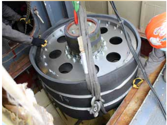
Figure 2. The new gear is lowered through the soft patch with just millimetres to spare.
