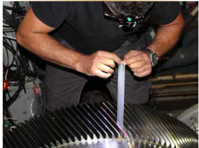
Figure 5. The meshing contact pattern is transferred from the port pinion gear onto sticky tape, which will then be stuck down onto a sheet of paper to be kept as a record.
