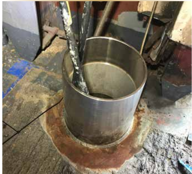
Figure 4. An uncoated stainless-steel sleeve welded to the mild-steel deck of a Halifax-class frigate.
