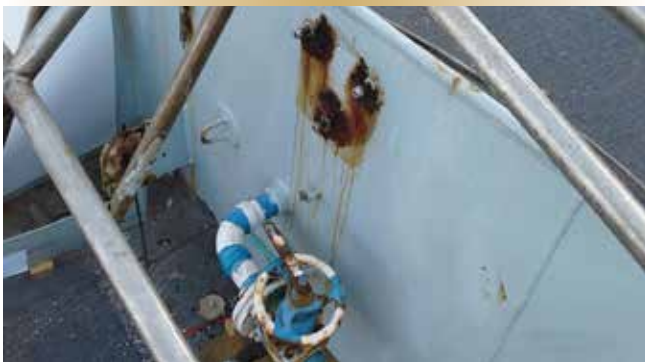
Figure 5. Dissimilar metal connections on the weather deck of a frigate.
