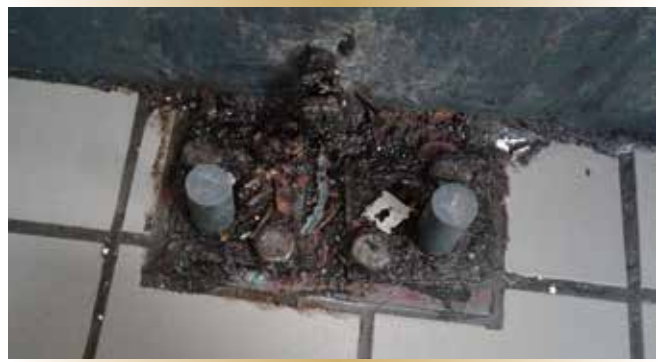
Figure 6. A severely corroded galley appliances connection.
