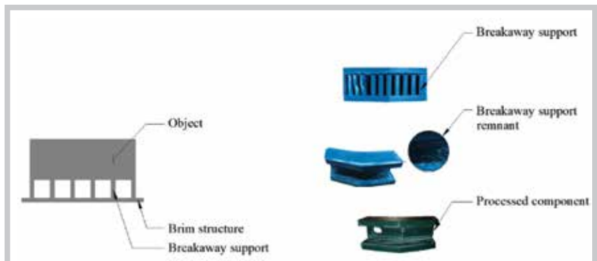
Figure 5. Breakaway Support Structure by PLA.
