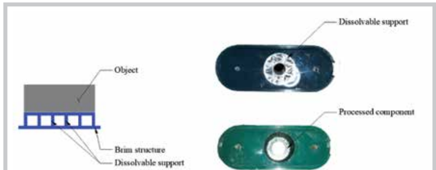
Figure 6. Dissolvable support structure by PVA.
