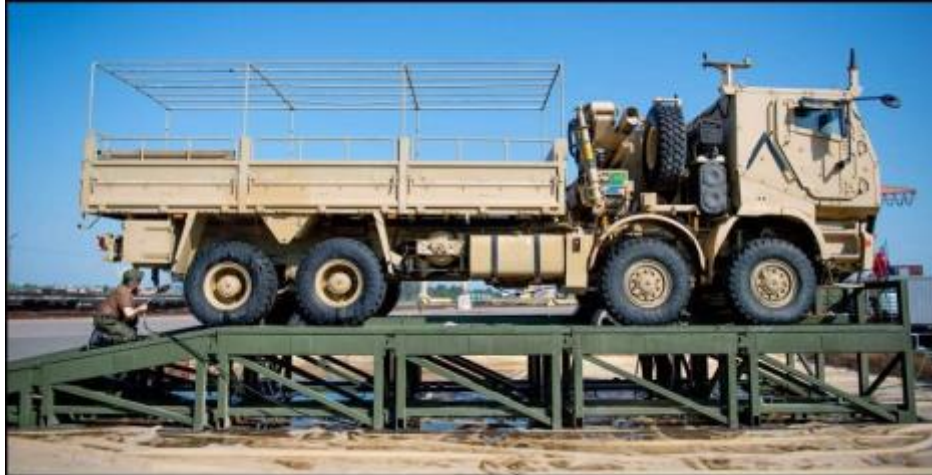
17 - A member of the IST deans an AHSVS up on vehicle ramps placed inside of a fuel berm. Photo Credit: Avr LeVasseur-Pearce, TFL Image Tech
