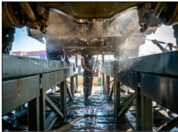
16 - A member of the PS Ops Platoon cleans the undercarriage of an AHSVS. Photo Credit: Avr LeVasseur-Pearce, TFL Image Tech
