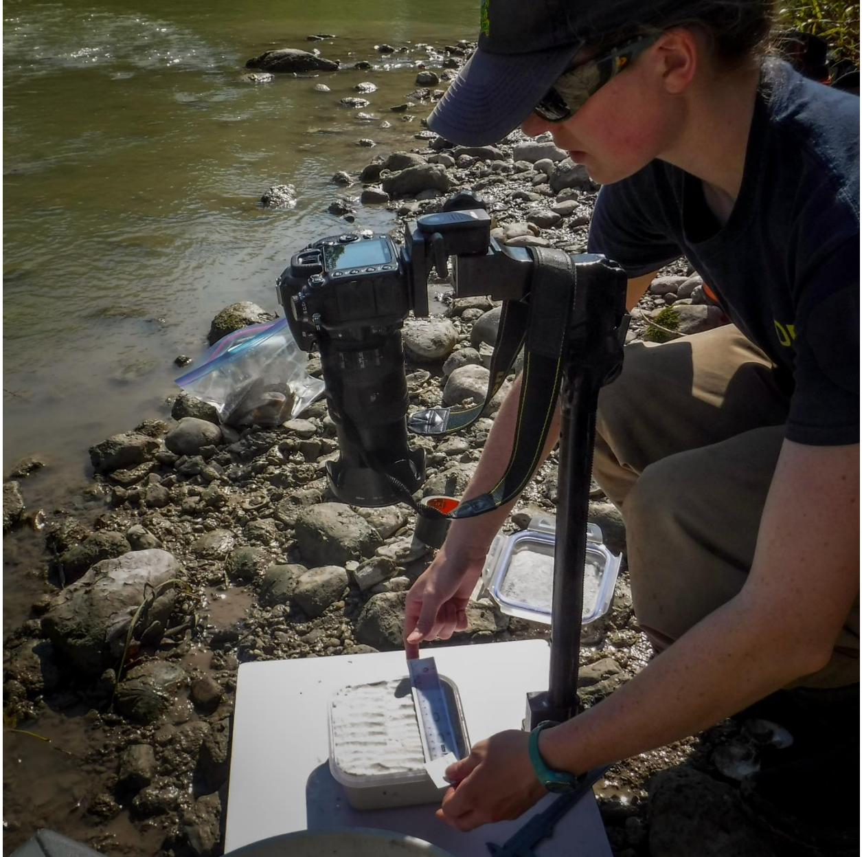
Figure 3. Photographic voucher setup demonstrating use of a copy stand. Note the sand container for positioning the specimen, presence of scale bar, and voucher label. Natural daylight allows for good colour rendition of the photographed specimens; reducing excess shading during sunny weather also yields better imaging. See Digital Voucher section for recommended details of voucher label.
