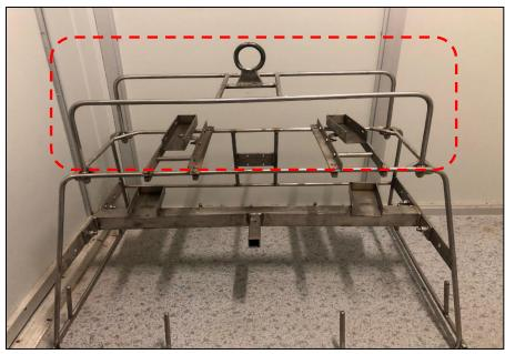
Figure 13. Removable guard (dotted box) for the lighting system attached to the main frame.
