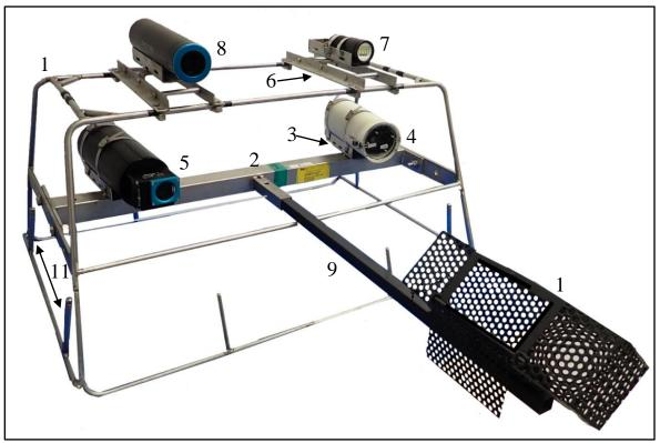
Figure 2. BRUV system and its components. 1= Main frame, 2= Camera bar, 3= Camera housing mounts, 4= Coastal housing, 5= Deep water housing, 6= Light mounts, 7= Dive light (coastal lighting), 8= Light housing (deep water lighting), 9= Bait arm, 10= Bait cage, 11= Sinker mount (not visible). Note: both configurations of the BRUV system include two coastal camera housings and two dive lights (coastal configuration), and two deep water housings and light housings (offshore configuration).
