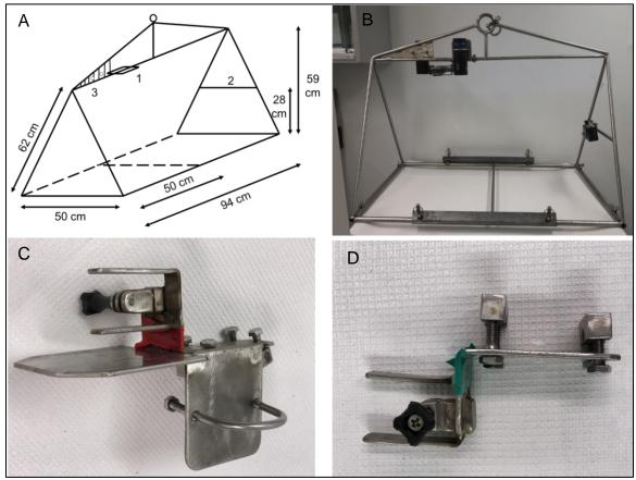
Figure 18. Deposited camera system (DPC) (A) diagram; (B) camera including removable camera mounts; (C) removable bracket for one of the two dive lights; and (D) mount for the tilted camera. In photo (A), 1 indicates the position of the vertical camera mount, 2 indicates the horizontal mounting bar for the tilted camera and 3 indicates the mounting bracket for the second dive light.
