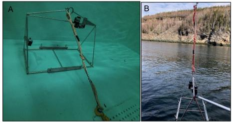
Figure 20. (A) A rigid, stainless steel rod measuring one metre in length runs along the rope, from the DPC system to the hook. It rests on the bottom in the water and (B) is shown in operation when attached to the hook of the boat, which prevents it from dropping into the quadrat or breaking the camera.
