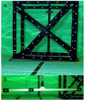
Figure 21. (A) Cube and (B) SeaGIS calibration bar.
