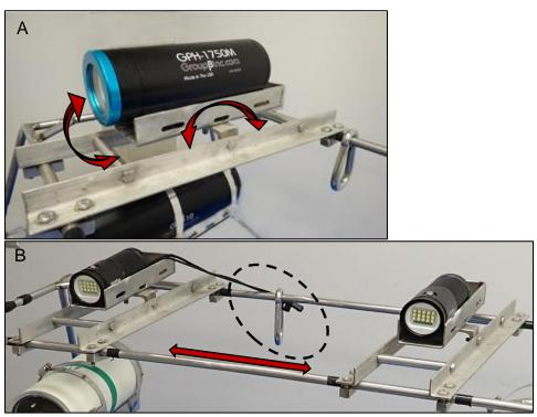
Figure 8. Positioning of lights and their mounts on the BRUV frame (A) for the deep water system and (B) for the coastal system. The arrows indicate possible adjustments. The dotted line in photo B indicates the safety knob.
