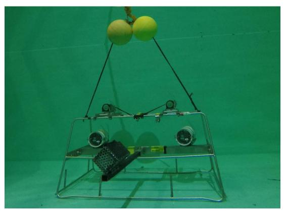
Figure 1. Baited stereoscopic underwater video system for sampling in coastal environments (0-100 m at chart datum).
