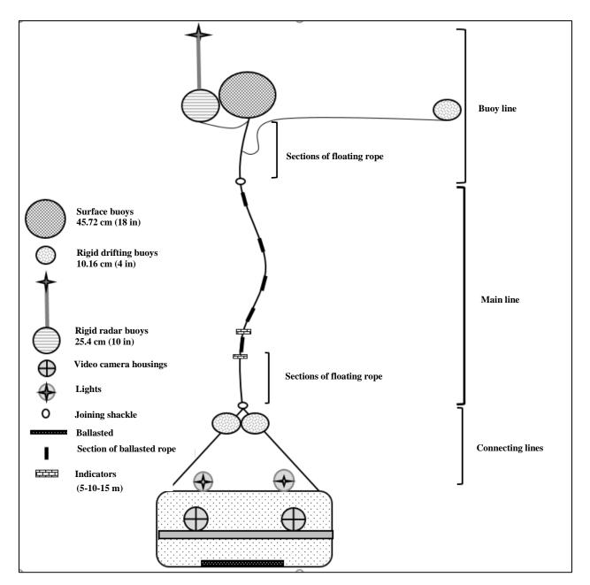
Figure 10. General diagram of the BRUV set systems
