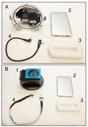
Figure 3. Camera system components (A), SeaGIS coastal housing (B) and GroupBinc Benthic 3 deep water housing. 1 = GoPro camera and viewport, 2 = external power source, 3 = support to stabilize the external battery, 4 = cable with USB-C connector at a 90° angle on the camera end (not visible) and USB-A connector on the power source end.
