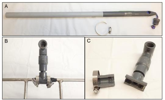
Figure 15. (A) Lowell TCM-1 current meter, (B) current meter installation mount on the BRUV frame, and (C) mount off the frame.
