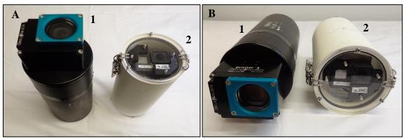
Figure 4. Benthic 3 (camera) and GPH10 (battery) housings used in deep water (< 1750 m) (A1 and B1), and SeaGIS housings used for coastal environments (< 150 m) (A2 and B2). The side view (A) illustrates the camera compartments, and the front view (B) illustrates the viewports and camera positioning.
