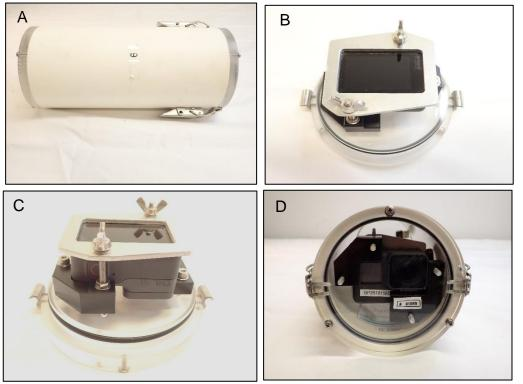
Figure 5. GoPro camera attachment and positioning mechanisms in SeaGIS coastal housings. Side view (A) with the positioning line to ensure the fixed position of the housing on its mount, interior view (B) (inside of the viewport) illustrating the camera attachment mechanism, side view (C) and front view (D) of the viewport.
