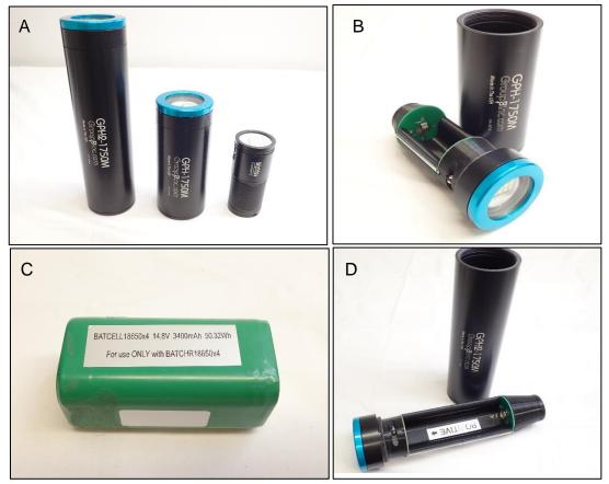
Figure 7. BRUV lighting system including (A), from left to right, the modified lights in the GPH 2 (long) and GPH 1 (short) deep water housings and a Bigblue VTL7200 light used in coastal systems; (B) inside view of a modified light in the GPH 1 housing; (C) Bigblue battery used in all light models; and (D) inside view of a modified light (dual battery) in the GPH 2 housing.
