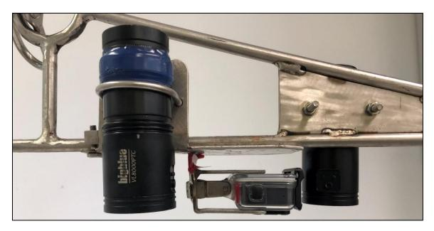
Figure 19. A lighting system with two dive lights installed on either side of the top camera to light up the quadrat.
