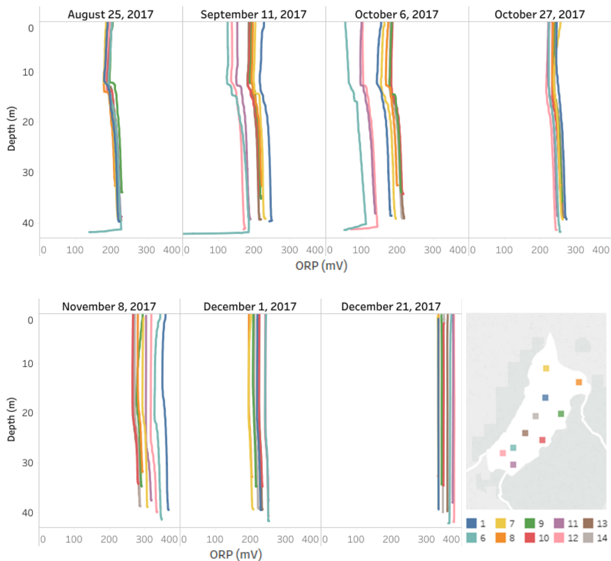
Figure 7. Depth profiles of redox potential (ORP) for each sampling day in 2017, with each DFO Water Monitoring Station represented by a colour.
