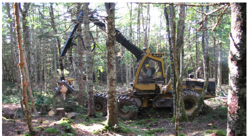
A "single-grip" harvester equipped with eco-tracks that limit damage to the forest floor selectively removes trees in a forest. Thinning the forest permits more light to penetrate the stand, encouraging faster regeneration of "climax" species such as white pine, red spruce, and yellow birch.
