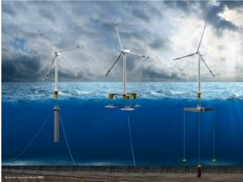
Figure 2.3.1: Offshore wind floating substructure designs: spar buoy (left), semisubmersible (middle), and tension-leg platform (right) [24]
