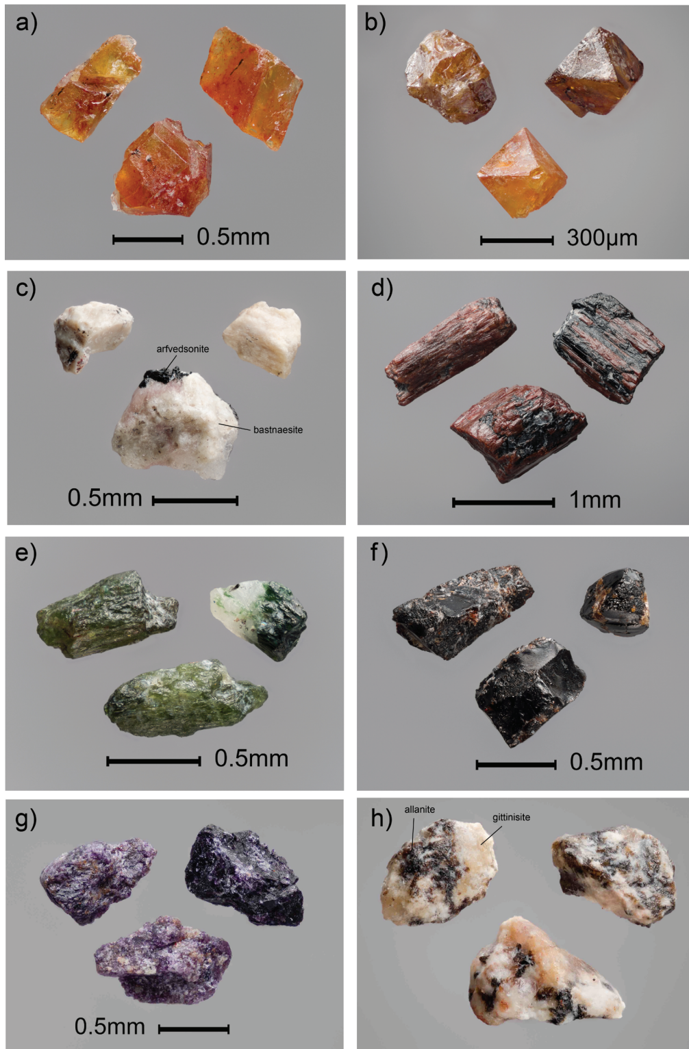
Figure 21. Colour photographs of selected indicator minerals from bedrock or from till samples overlying and down ice of the Strange Lake rare-earth element deposit: a) orange monazite; b) orange-brown octahedral pyrochlore; c) white bastnaesite grains; d) reddish brown to black fibrous arfvedsonite; e) dark green acicular aegirine; f) black chevkinite; g) dark purple fluorite; h) dark brown allanite intergrown with white gittinsite. Photographs by Michael J. Bainbridge Photography. From McClenaghan et al. (2019)
