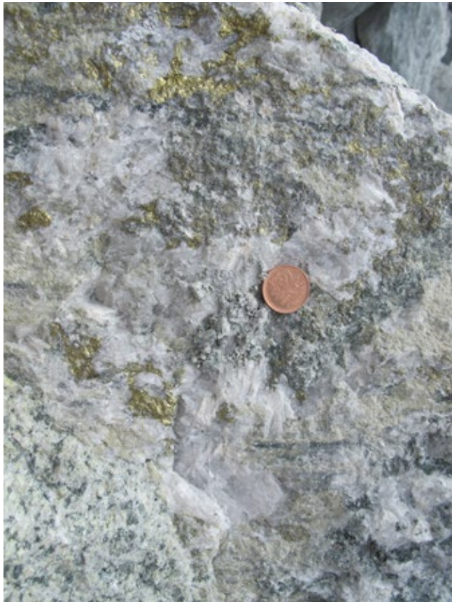
Figure 31: Supergene mineralization of native copper, chalcocite and hematite at New Afton mine, south central British Columbia
