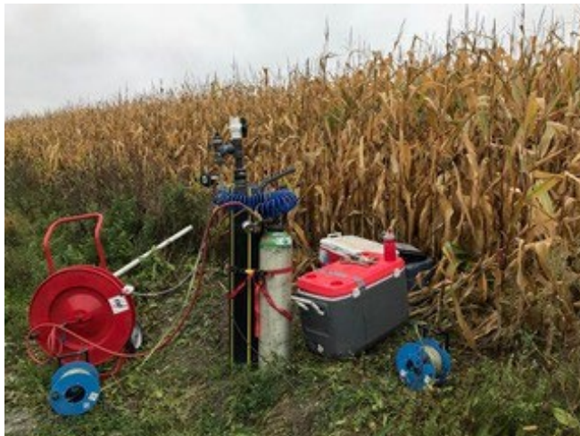
Figure 20: Drilling operations with a portable dual-rotary rig for the installation of a well in an unconsolidated aquifer near Ottawa, ON. The drilling technique was adapted to allow high-resolution profiling of hydraulic properties in granular aquifers
