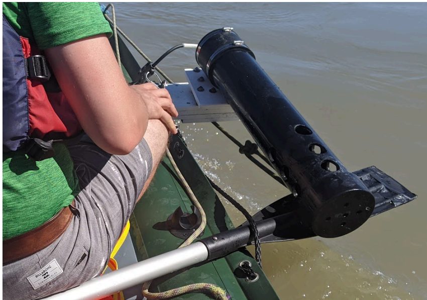
Figure 9: Housing for water quality sonde, currently being held up by paddle for travelling quickly between observation sites. The hinged assembly allows it to lower into the water during measurement. Photograph by M. Hodul. NRCan photo 2022-310.
