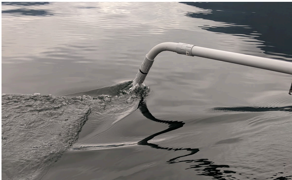
Figure 8: the water-facing spectrometer head, housed in an angled grey PVC pipe, used to shade the water being observed, to prevent water reflection. Notice the black line on the pipe near the water, indicating the location of the end of the spectrometer, which must remain above water during measurement. Photograph by M. Hodul. NRCan photo 2022-309.
