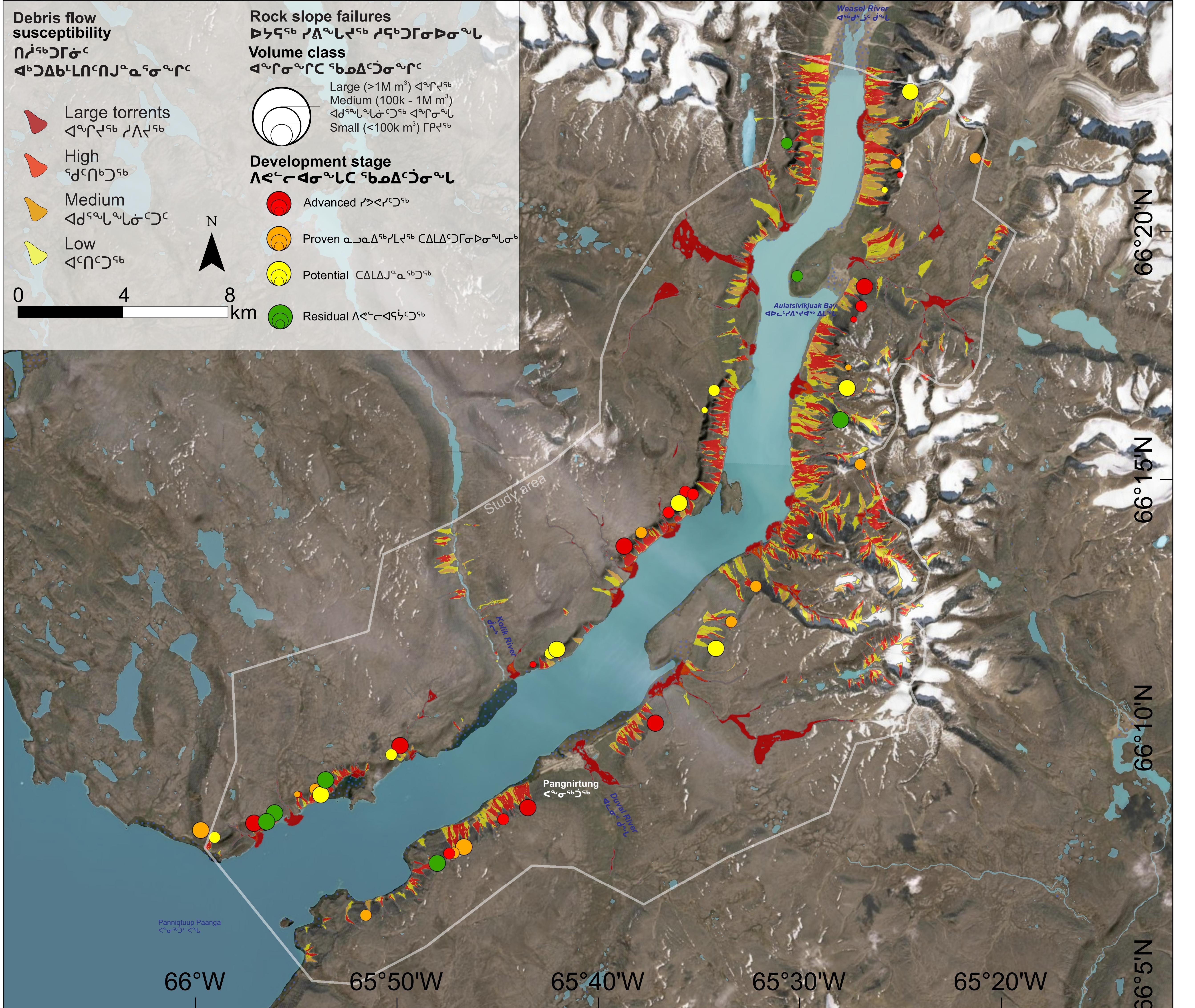
Figure 1. Debris flow susceptibility and inventory of rock slope failures in Pangnirtung Fiord.
