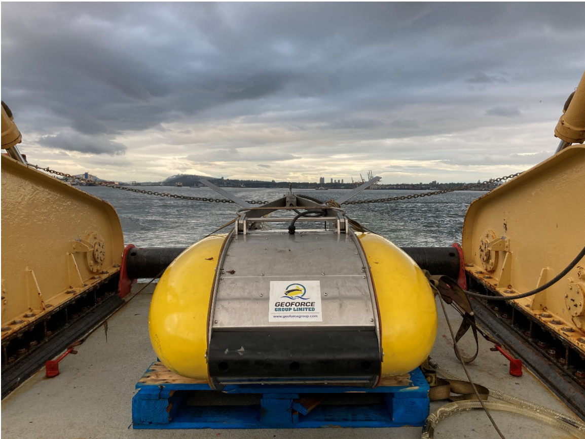
Figure 3. Photograph of the Geoforce Deep-tow System on the aft deck of the Vector, below the A-frame. Photograph by K. Douglas. NRCan photo 2021-664.
