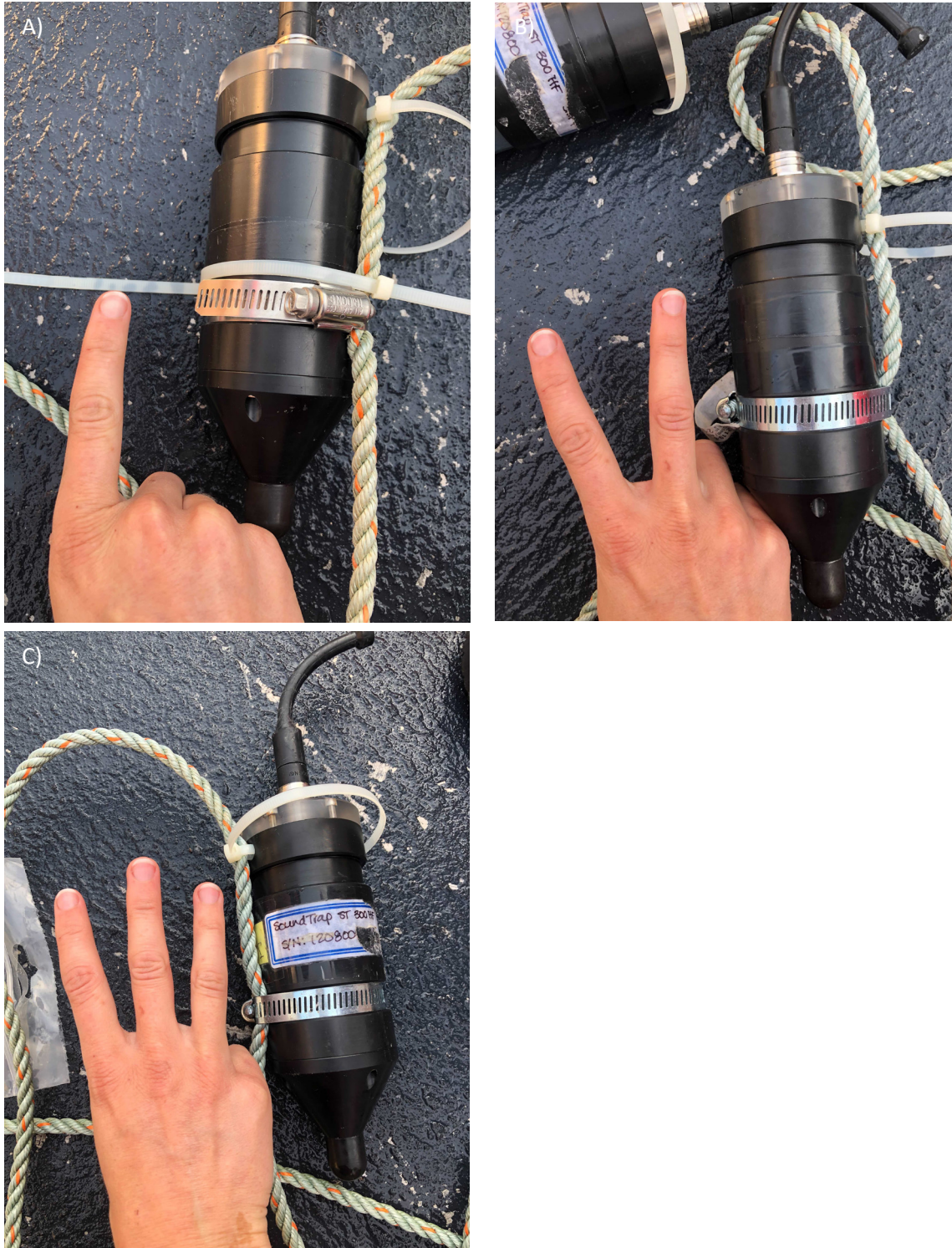
Figure 4. Photographs of the three Jasco sound trap hydrophones (Juanes Lab, UVic) used in the Saanich Inlet sound exposure level experiment. Depths deployed were A) 5 m = 1 band of black electrical tape, B) 10 m = 2 bands of black electrical tape, C) 15 m = Juanes lab label. Photographs in this figure used with permission, courtesy of Desiree Bulger, Malahat Nation.
