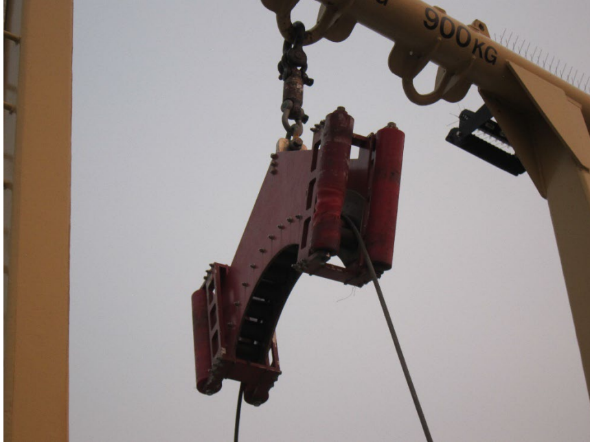
Figure 9 - Roller Block in operation
