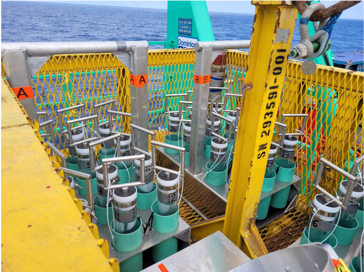
Figure 8: Quivers loaded with empty push cores inside the work basket ready for deployment (Courtesy of D. Gittins).
