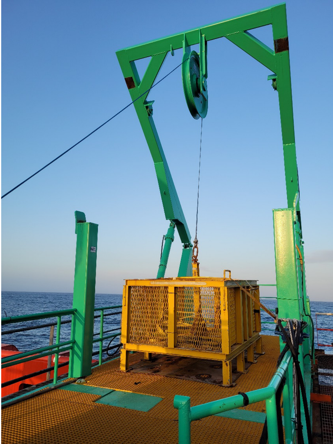
Figure 9: Work basket (empty) and work basket A-frame located on the mezzanine deck of the Atlantic Condor (Courtesy of D. Gittins).
