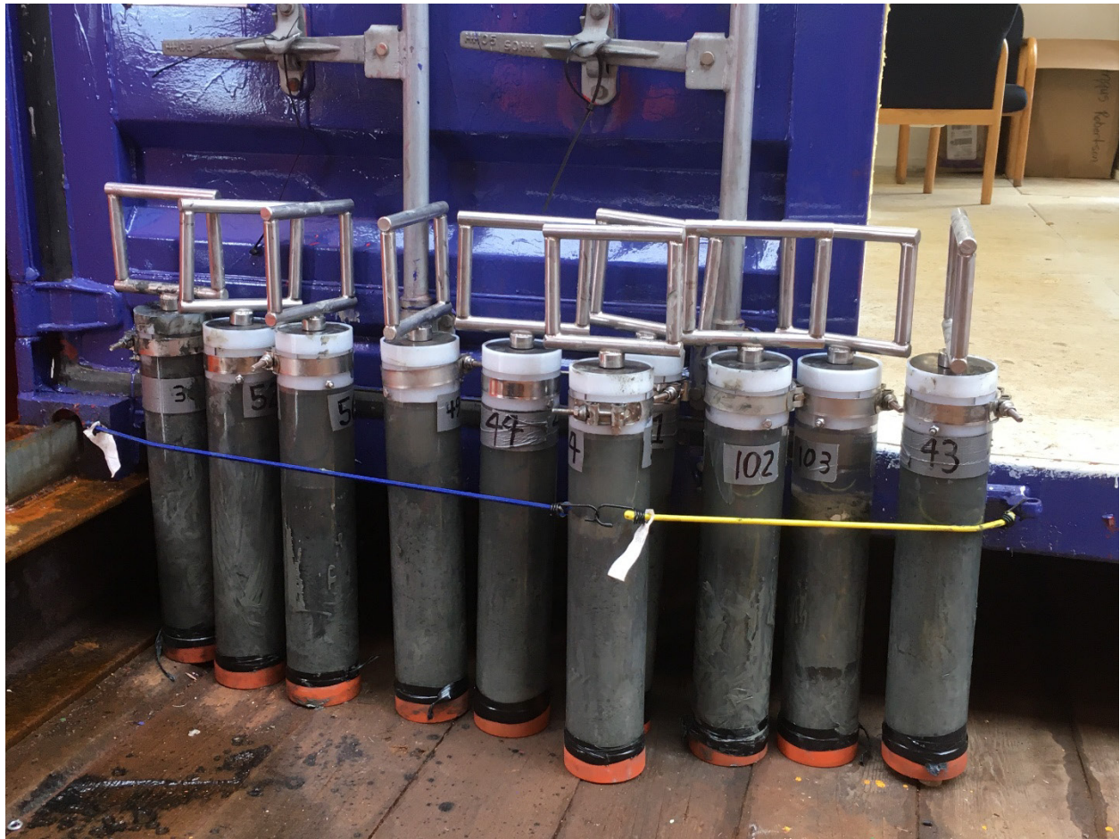
Figure 7: ROV push cores on deck following sediment collection. Each clear plastic tube is 50 cm long and has an internal diameter of 8.89 cm (Courtesy of A. Chakraborty).
