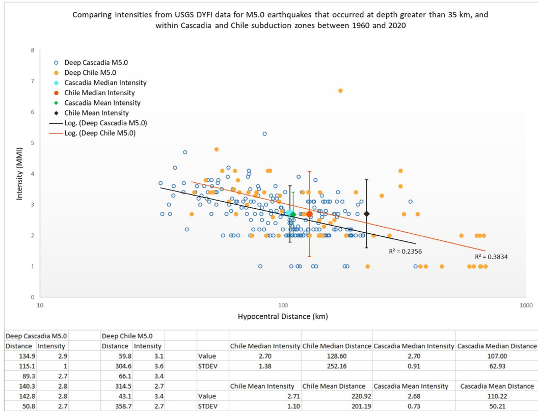
Figure 7: An example of a combined plot with associated data, showing all Chile & Cascadia earthquake response values combined on one graph. The table below the plot, shows the calculations use for the mean and median.
