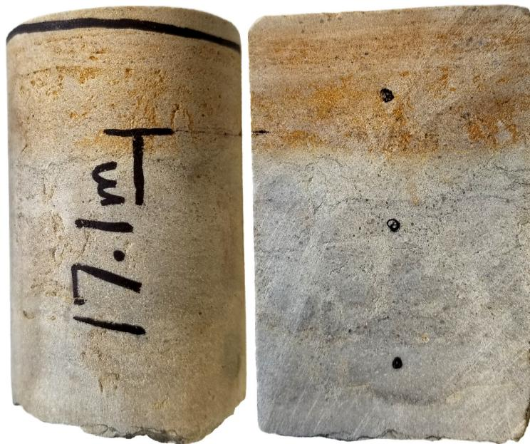
Figure 7: Example of split drill core for used for pXRF, fusion and 4-acid laboratory analysis. Outer curved surface (left) and inner cut surface (right). The three black dots on the right core image indicate where pXRF analyses were obtained. A core depth of 17.1m is marked on the core, which corresponds to a wireline depth of 16.7m. Core sample length 7.0cm. Photographs by L.C. Olson. NRCan photograph DB numbers: 2022-307 (left image); 2022-308 (right image).
