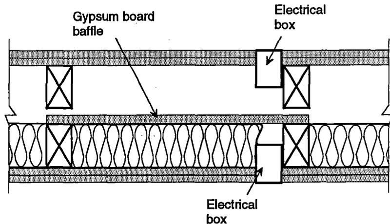
Table 6: Comparison of the effectiveness of a gypsum board baffle in a double stud wall with and without absorption to reduce the effect of poorly located electrical boxes. The sound insulation is expressed in terms of the STC.
