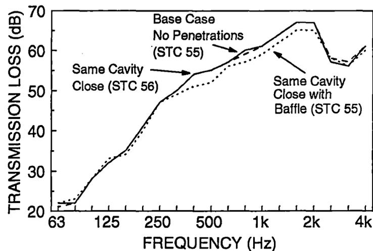
As shown in Figure 13, the performance of the wall without the baffle was better. If several of this type of baffle were used in a wall, then it is probable that the sound insulation would be affected even more than the small reduction in STC observed here.
