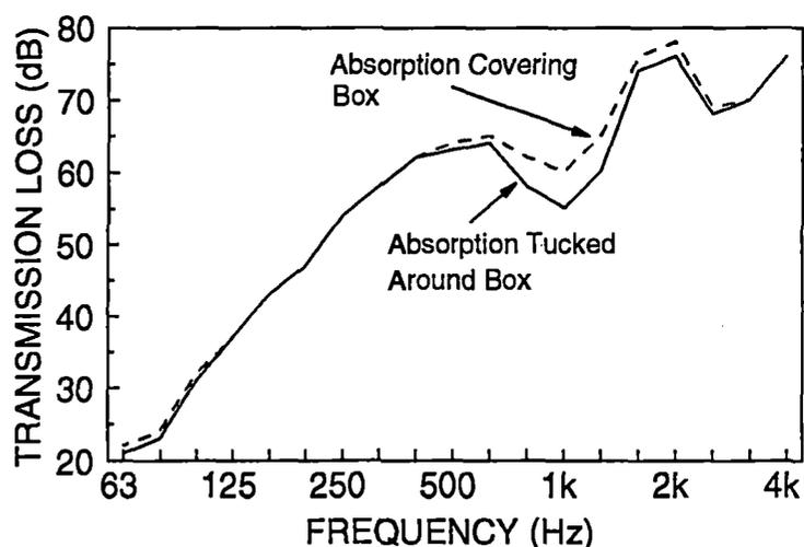
Cavity absorption reduces the effect that poorly placed electrical boxes have on the sound insulation of a party wall. Where possible, the batt insulation should not be displaced around the electrical boxes as this will reduce the effectiveness of cavity absorption.
