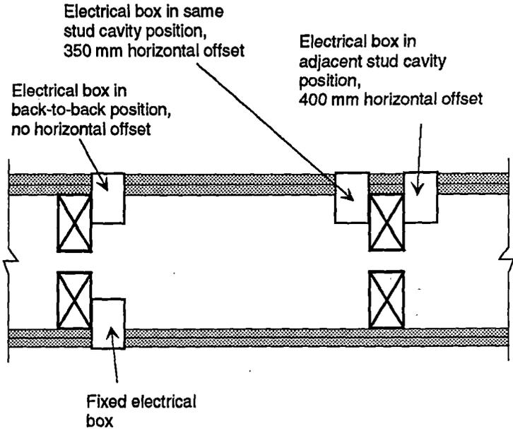
Figure 1(b): Positions of the electrical boxes in the double stud wall. This construction was the same as in Figure 1(a), but with 90 mm glass fibre batt displaced around the electrical boxes in the stud cavity (see also Fig.4).
