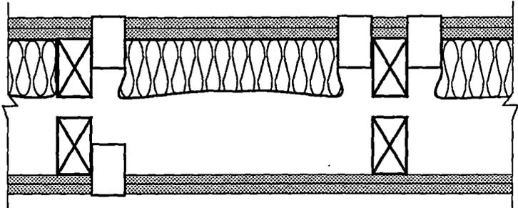
Figure 1(c): Positions of electrical boxes in the double stud wall. This construction was the same as in Figure 1(b), but with 90 mm glass fibre batts installed against the studs and between outlets.
