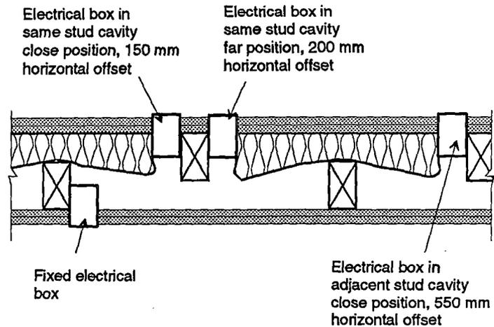
Figure 3: Positions of electrical boxes in the single stud wall. The single stud wall was constructed as follows:
