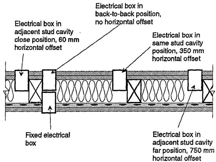
Figure 4: Sketch of a vertical wall section showing the insulation 'displaced' around each electrical box. Note that boxes are exposed to adjacent airspace behind the box, or to each other in case of back-to-back outlets.
