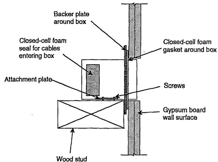
The sound insulation for standard metal boxes without any treatment was compared to that with the plastic boxes, when installed in the double wood stud wall without cavity absorption (a sensitive case).
