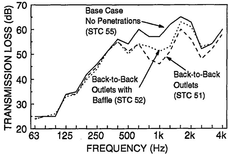
However, when there is significant cavity absorption the amount of reverberant energy is very low and reducing the direct energy with the use of a baffle will be most effective. This is demonstrated in Figure 11.
