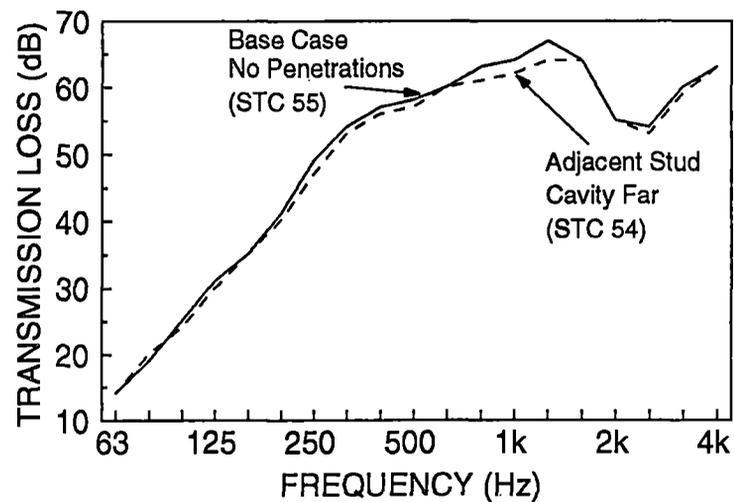
Figure 14 shows the measured sound insulation (with and without electrical boxes) of a wall with one gypsum board surface mounted on resilient channels. The electrical fitting and the faceplate were screwed firmly against the gypsum board.
