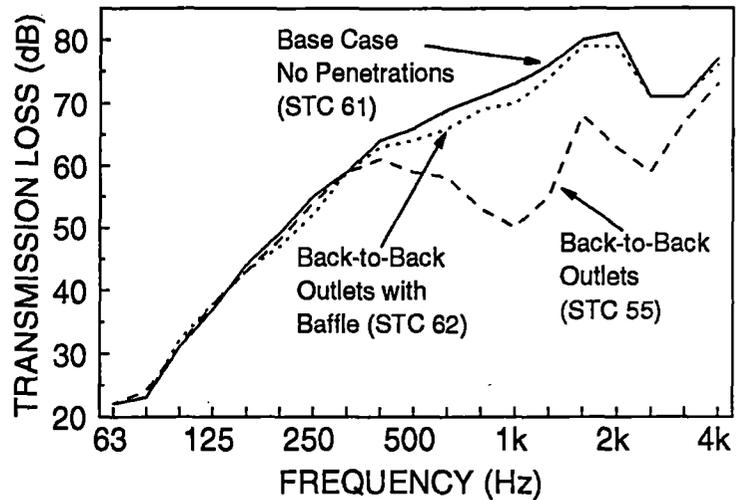
For double wood stud constructions having cavity absorption, the baffle is the most effective treatment. However, it is among the least effective if there is no cavity absorption.
