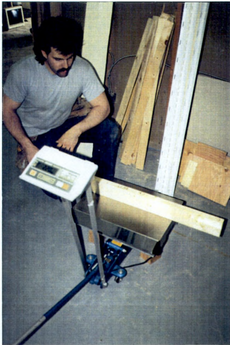
Photo 5 Weighing of text panel components with weigh scale cart.
