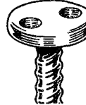
Drilled spanner Tamper-resistant. Can be used with magnetic drivers that grip the whole head.
