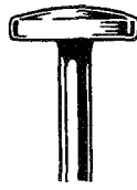
Pan Wide head allows great clamping strength. Not very attractive, so usually used where not seen.
