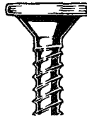
Water Similar to bugle head, but wider and thicker. Good for soft materials.
