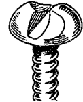
One-way Tamper-resistant. Can be installed with regular screwdriver but removed only by special tool.
