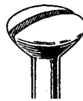
Slotted Useful now mostly on antiques, where other options would look out of place.
