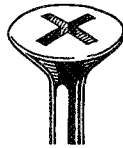
Phillips Cross-drive recess has tapered, flat-bottomed slots. Named for 1935 inventor, Henry M. Phillips.
