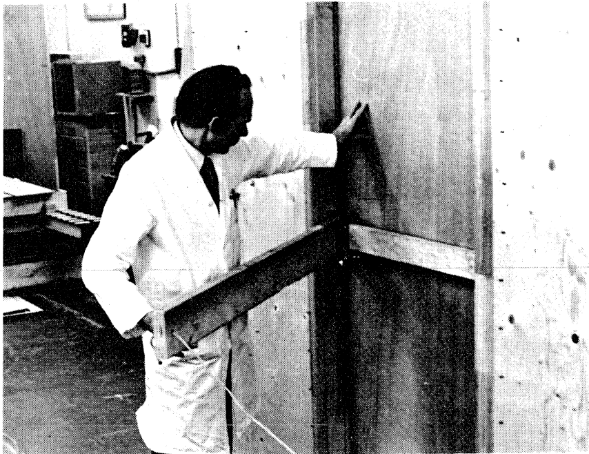
Figure 2. Apparatus for jamb/wall stiffness test.
