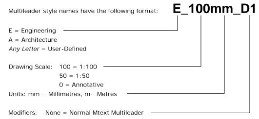
D1 = Multileader with Detail Callout Block (D2, D3, etc. for alternate Detail callout Blocks)
