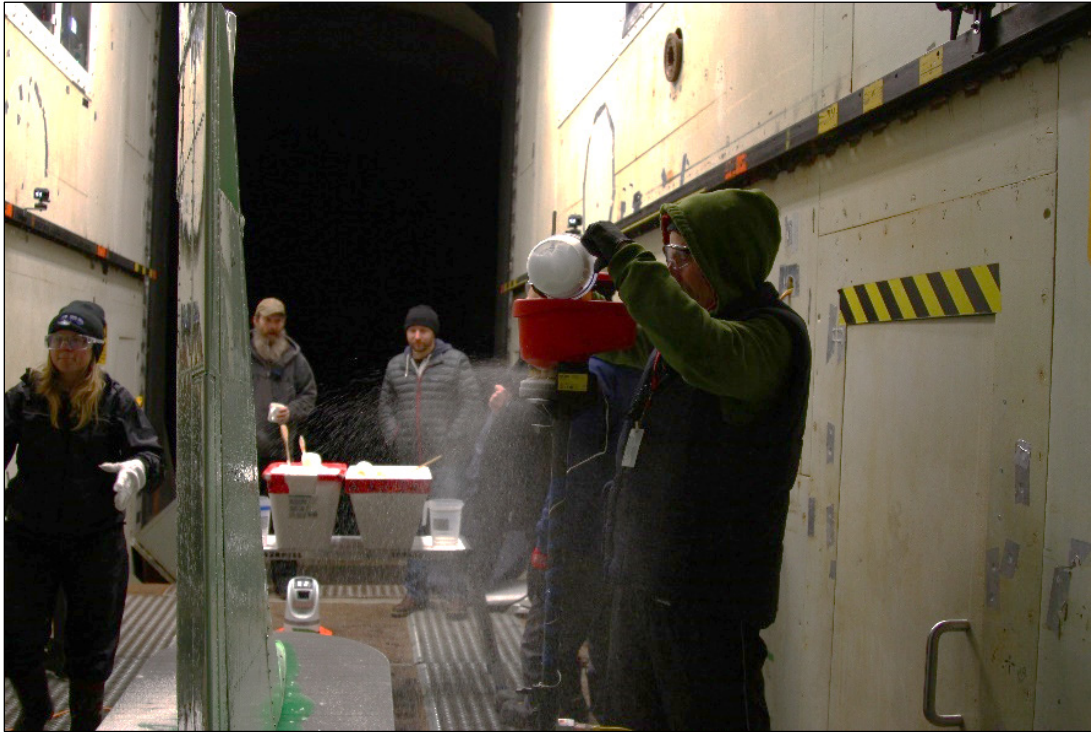
Photo 2.9: Ice Pellet/Snow Dispenser Operated by APS Personnel
