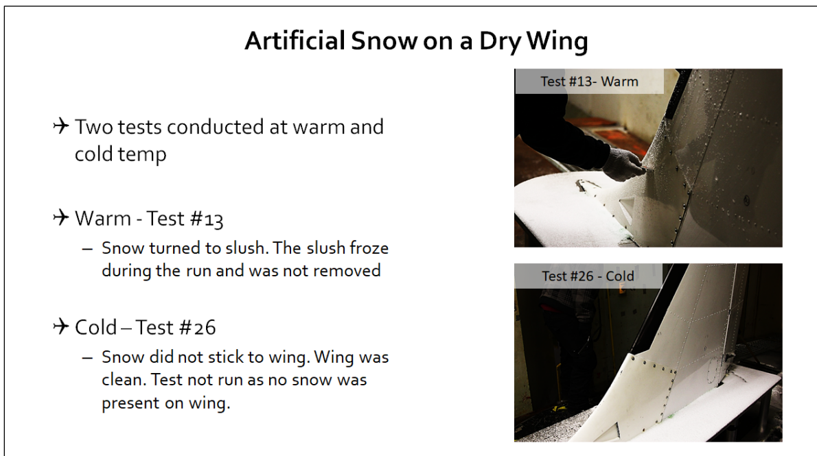
Photo 6.10: Artificial Snow on a Dry Wing
