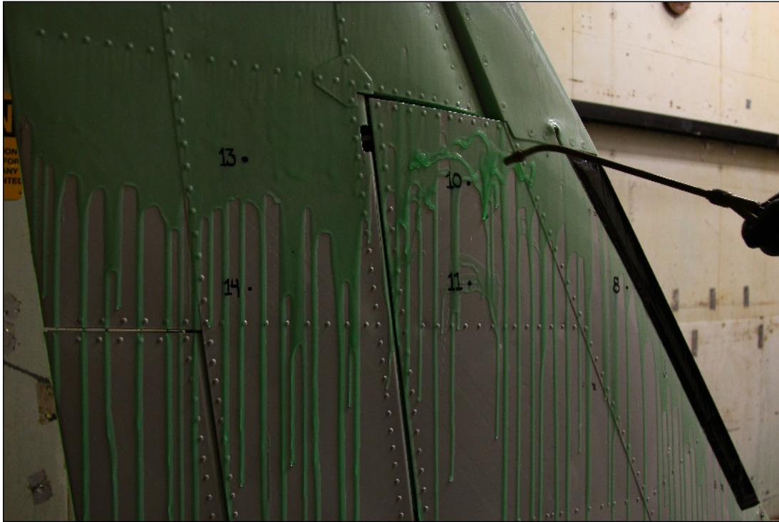
Photo 2.15: Garden Sprayer Hand-Held Wand Applying Fluid
