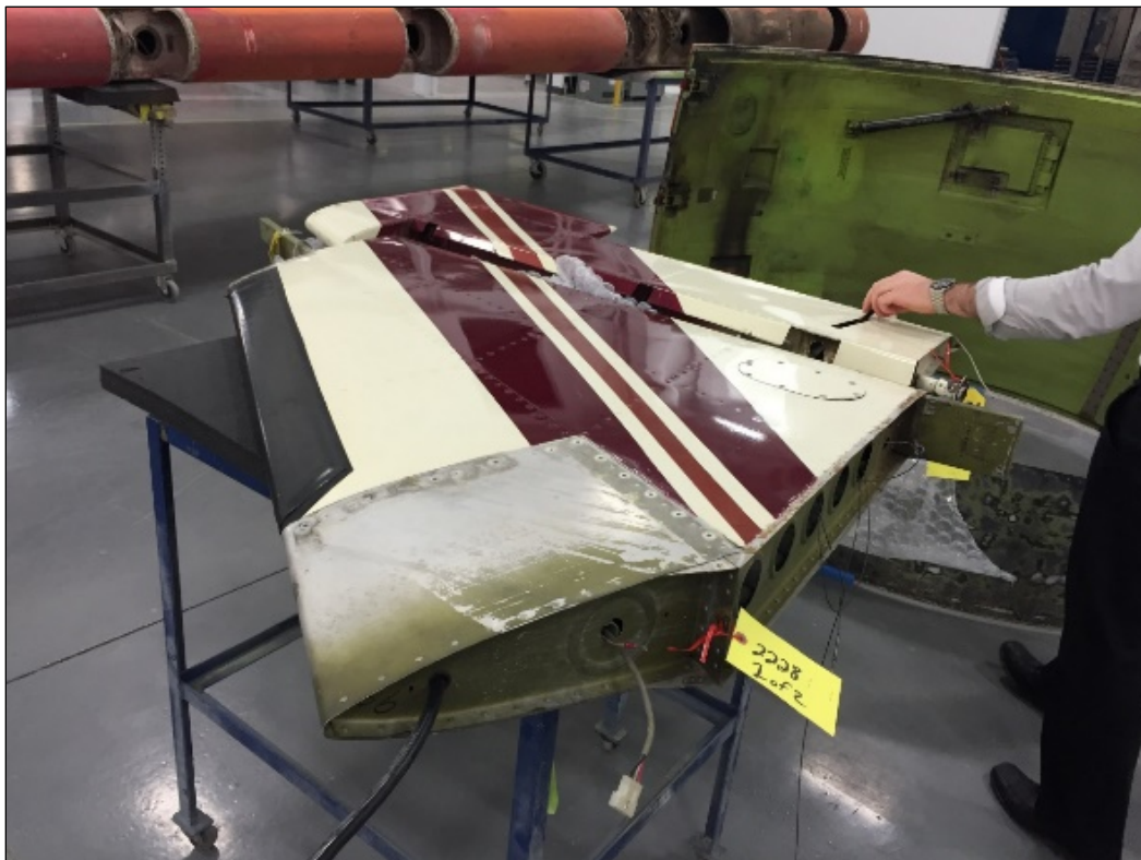
Photo 2.4: Salvaged Piper PA-34-200T Seneca II Vertical Stabilizer
