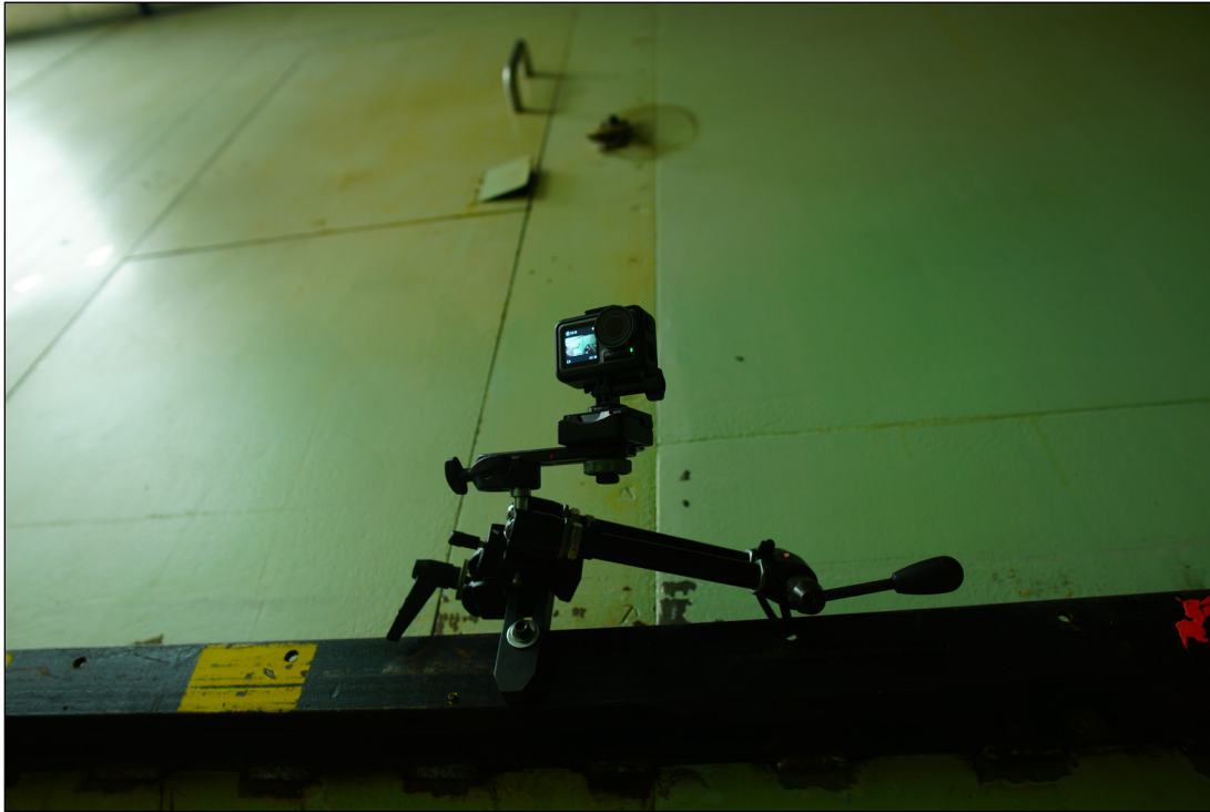
Photo 2.13: Osmo ® Video Camera Installed on Wall of Wind Tunnel
