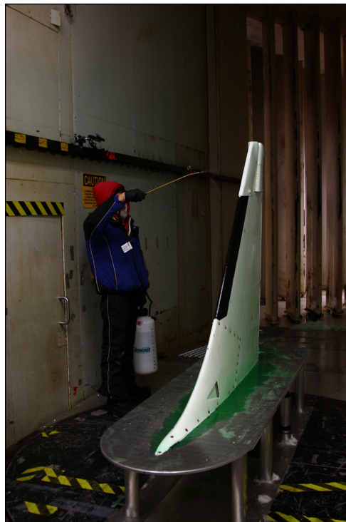
Photo 2.10: Simulating Freezing Rain with Garden Sprayer
