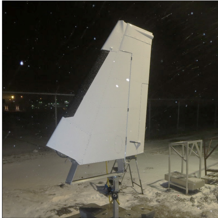
Photo 2.5: Vertical Stabilizer Mounted for Endurance Time Testing Outdoors
