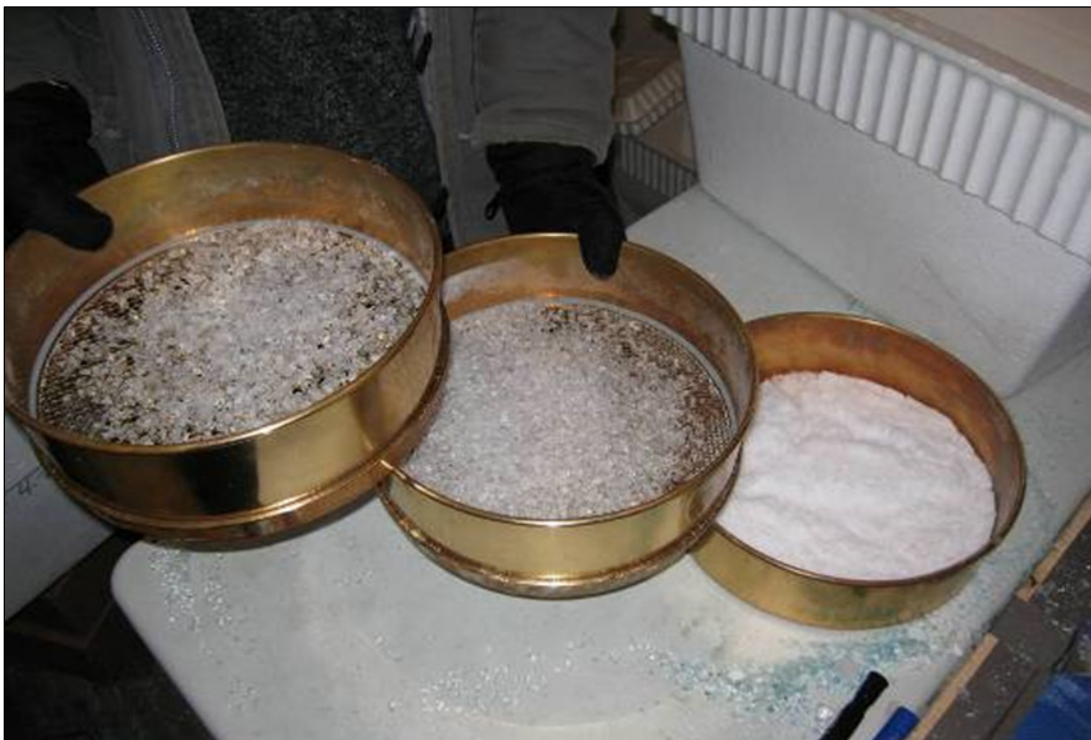
Photo 2.8: Calibrated Sieves Used to Obtain Desired Size Distribution
