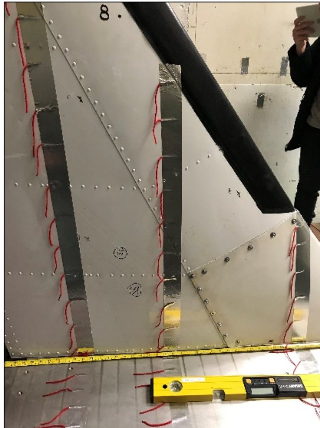
Photo 5.1: Tufts Attached to the Vertical Stabilizer Model Using Speed Tape
