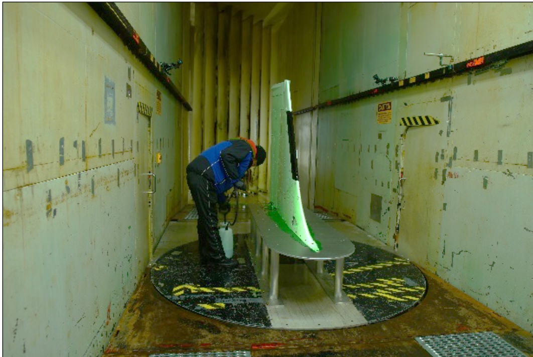
Photo 2.6: Vertical Stabilizer Mounted in the NRC IWT for Testing
