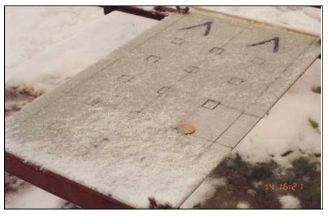
Photo 5.2 - Snow-Bridging Failure of Anti-Icing Fluid on an Aluminum Plate
