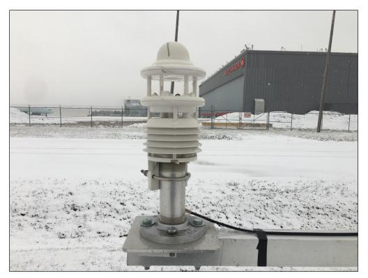
Figure 2.4: WS600 Multi-Parameter Weather Sensor
