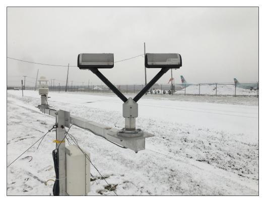
Figure 2.6: Parsivel<sup>2</sup> Disdrometer
