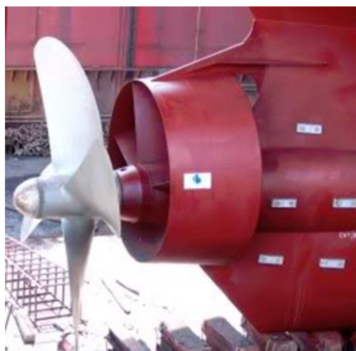
Figure 31. Typical installation of a Mewis duct wake equalizing devices (WED).
