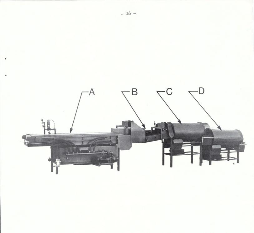
Figure 1. Fox lye peeling system. A. Caustic bath; B. "Reaction" conveyor; C. Peeling cylinder; D. Rinse cylinder.
