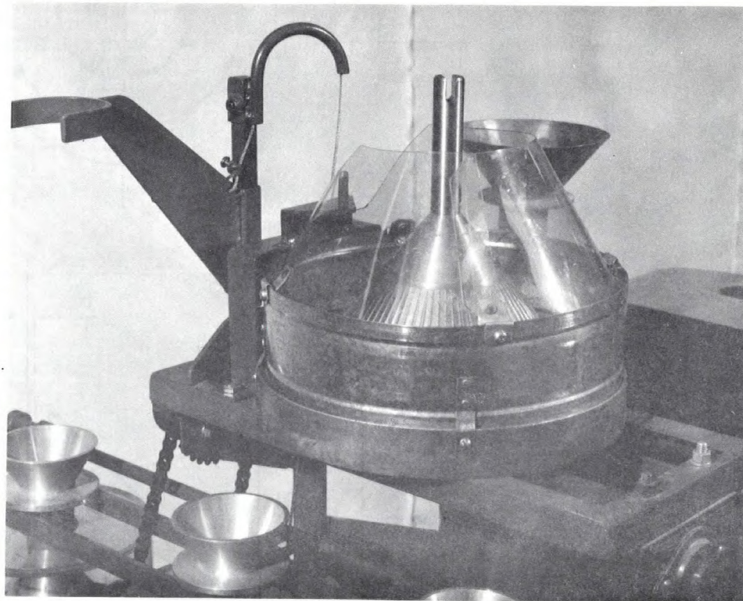
Fig. 1. B. View of modified cone showing drive post, sheet metal ring, plexiglass shield and reaction post.
