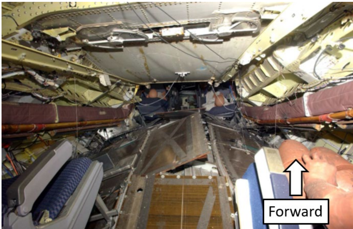
Figure 20. Photo of reduced habitable (survivable) space in centre cabin as a result of collapsed wing and intrusion of main landing gear structure during 2006 drop test (Source: U.S. Federal Aviation Administration, with TSB annotations)
