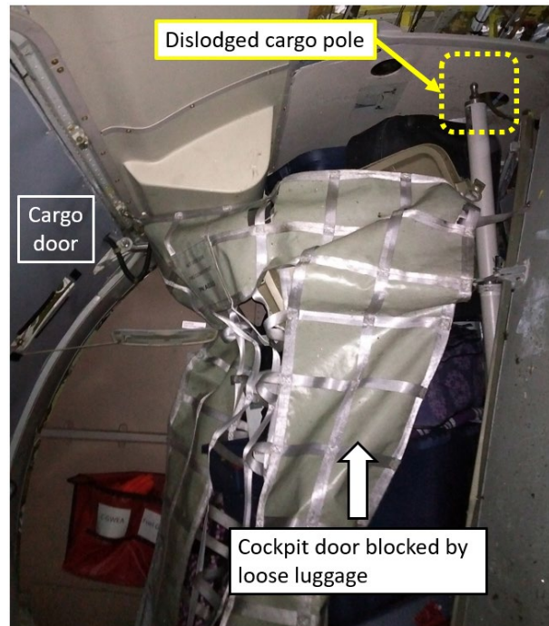
Figure 32. Main cockpit door blocked by loose luggage as a result of dislodged cargo pole (Source: TSB)
