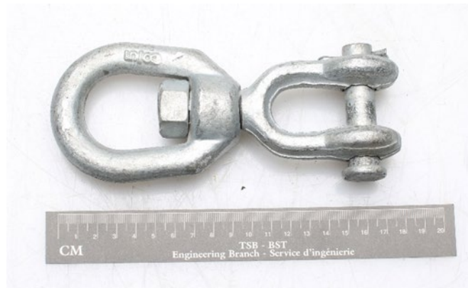
Figure 9. Photo of the Crosby G-403 jaw end swivel used in the occurrence (Source: TSB)
