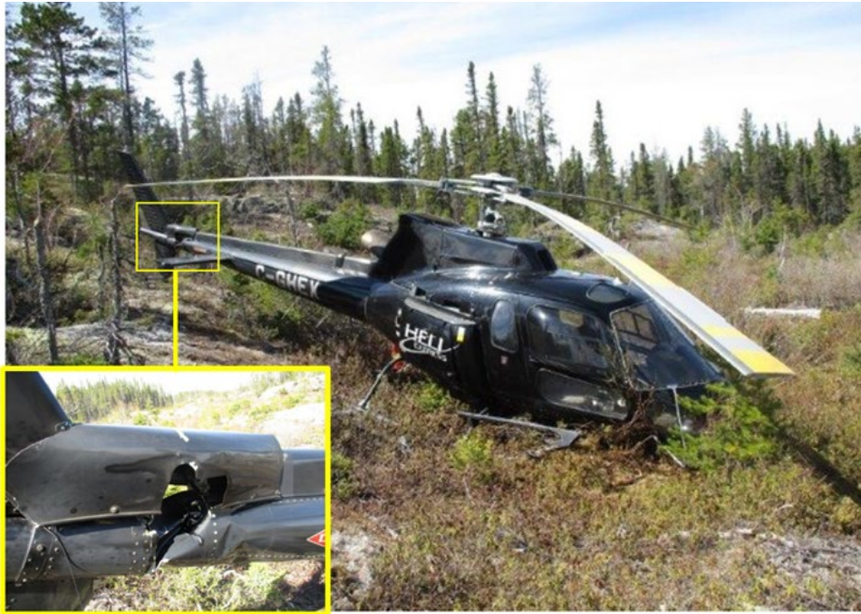
Figure 3. Photo of the wreckage, with inset image showing a magnified view of the damage to the tail (Source: Sûreté du Québec)
