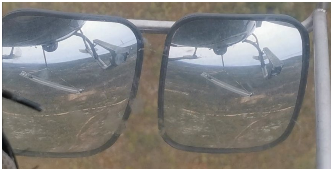
Figure 13. Images reflected in the helicopter's mirrors, showing the position of the platform while being carried horizontally, without a sling, during the test flight (Source: screen shot of a video filmed by the occurrence pilot during the test flight)
