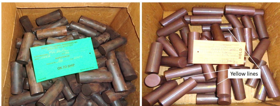
Figure 10. Pictures showing the shipments of conforming pins (left) and non-conforming pins (right) (Source: Bodycote, with TSB annotations)
