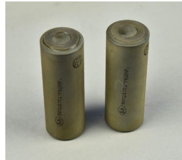
Figure 11. Example of 316 stainless steel pin on the left and H11 tool steel pin on the right (Source: Bell Textron Inc.)
