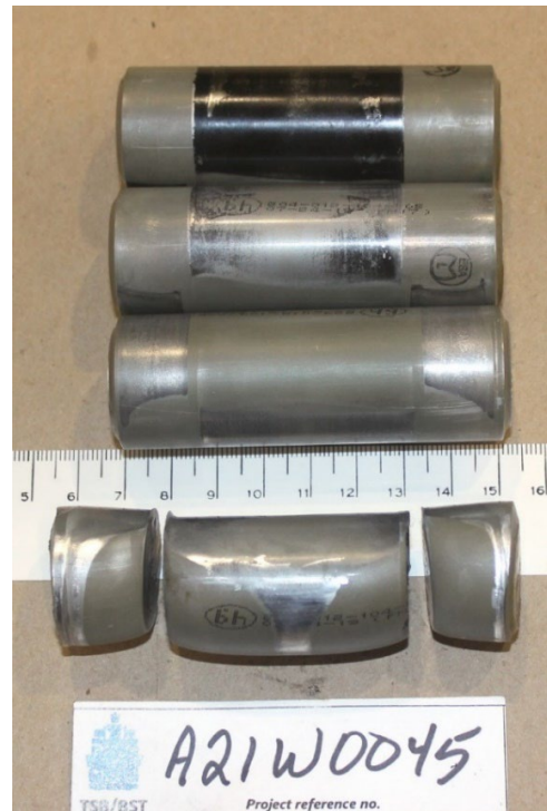
Figure 7. Photo of the occurrence helicopter's 4 main rotor hub strap retaining pins (Source: TSB)
