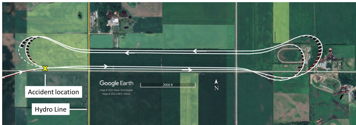
Figure 1. Actual (solid line) and estimated (dashed line) occurrence flight path based on GPS (global positioning system) data (Source: Google Earth, with TSB annotations)
