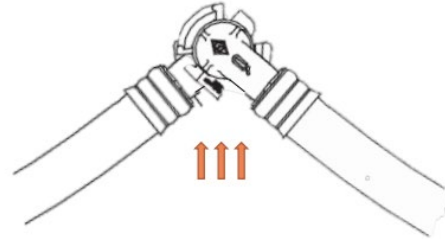
Figure 10. Coupled gladhand couplings in a peaked orientation due to upward force (Source: Y. Wang, "Brake System End Arrangement Tests," presented at the Railway Supply Institute Expo and Technical Conference, Fort Worth, Texas, 11–13 October 2022.)
