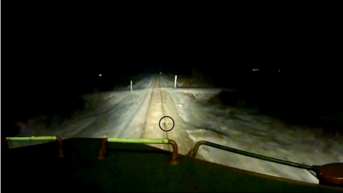
Figure 5. Still image captured from the forward-facing video camera on the head-end locomotive, showing a gap in the south rail (circled) (Source: Canadian Pacific, with TSB annotations)
