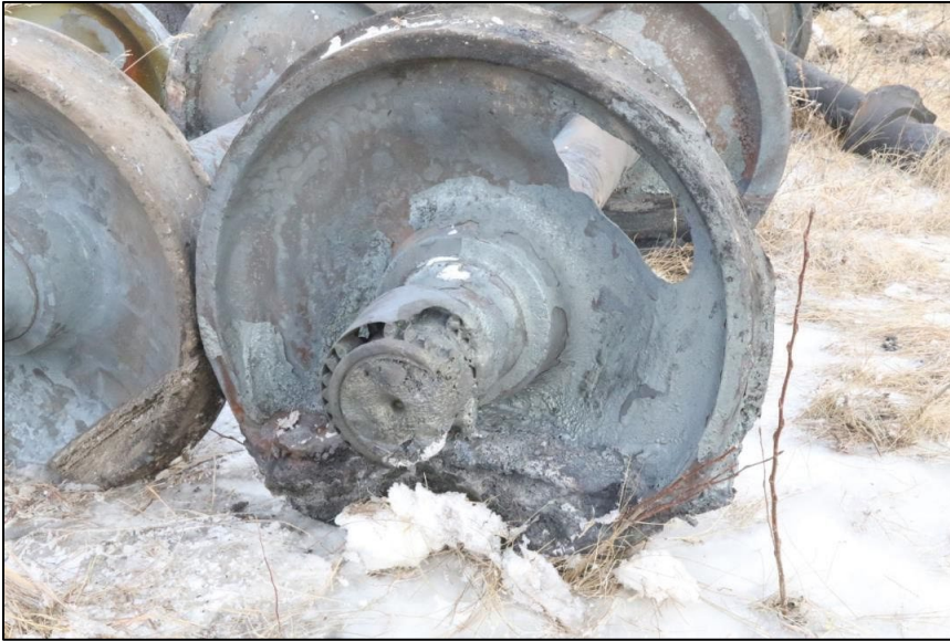
Figure 9. Unidentified melted wheel set from the fire (Source: TSB)
