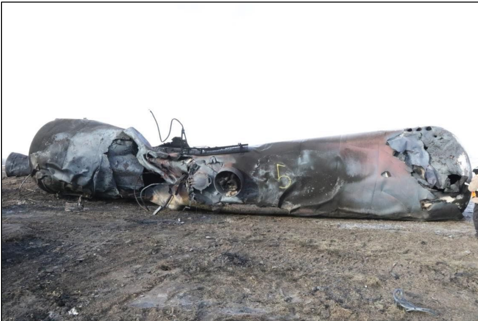
Figure 10. Severely damaged unidentifiable tank car with multiple breaches (Source: TSB)
