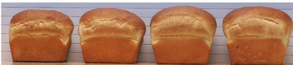
Figure 2 The Sponge and Dough bake test resulted in loaf volumes that increased as protein content increased.
