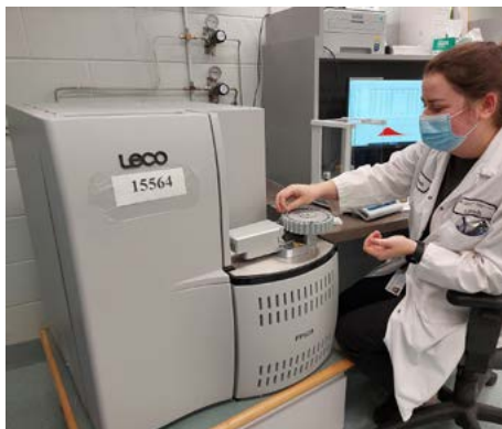
Figure 3 Equipment used for combustion nitrogen analysis (CNA).
