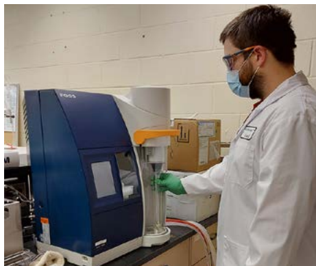
Figure 2 Measuring protein content using Kjeldahl analysis.
