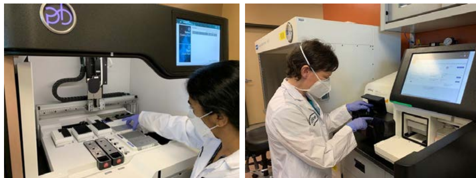
Figure 1 High-throughput robotic DNA sequencing equipment used for gathering whole genome information on microorganisms and grain crops.
