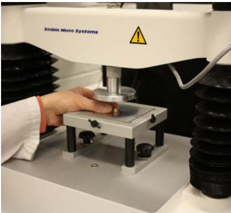
Figure 3 Texture analyzer used for determining the hardness of pulse seeds.
