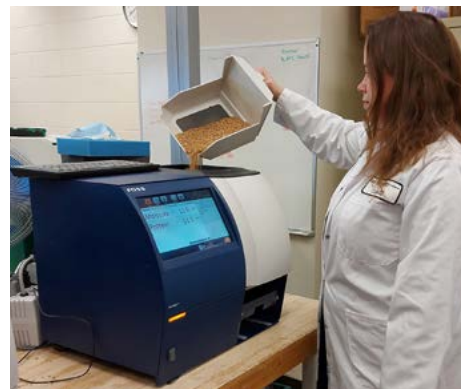
Figure 4 Near infrared transmittance (NIT) instruments used to predict protein content.
