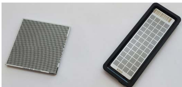
Figure 3 DNA arrays that allow for thousands of targeted DNA genotyping tests to be performed at once. Pictured above are a Takara SmartChip plate (left) and an OpenArray™ plate (right).
