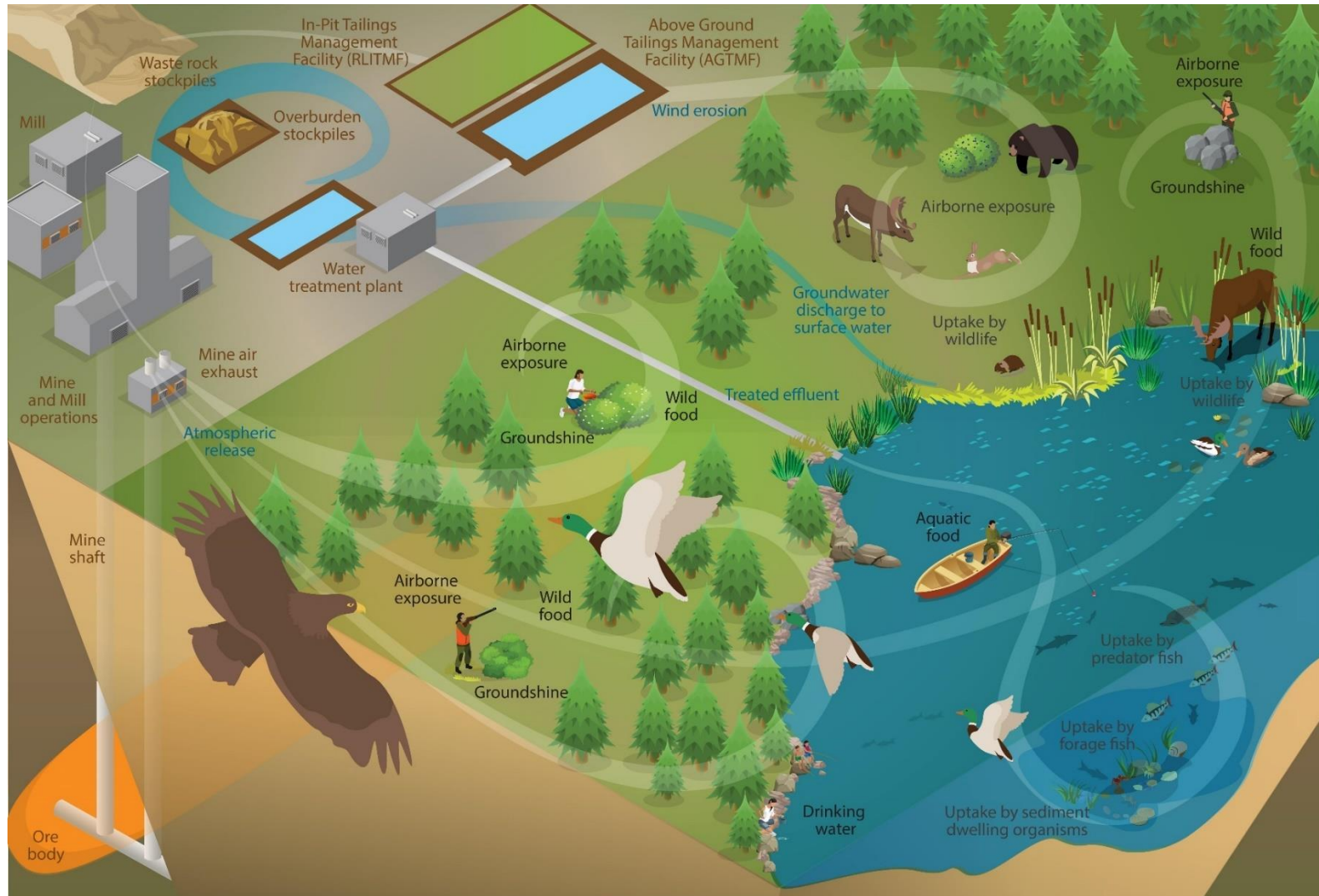
Figure 3.1. Conceptual model of the environment around the Rabbit Lake Operation
