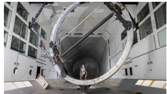
The rain-wind rig permits the study of stay-cable vibration on full-scale models
