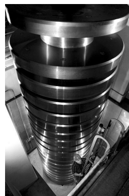
Stack of stainless steel weights in the 4.45 meganewton (approximately 454 000 kilogram-force) deadweight machine that the NIST uses to calibrate load cells.
