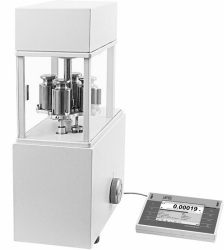
Radwag AK-4/2000 Automatic Mass Comparator (Radom, Poland).
