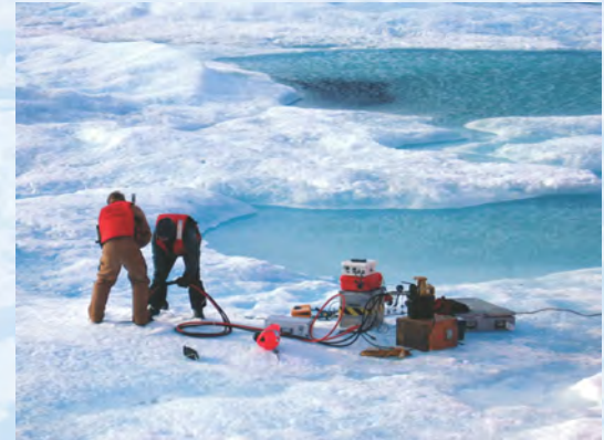
Measuring the strength of multi-year ice, as discussed in the section Growth and Ageing of Sea Ice .
