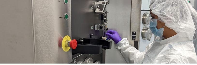
A biomanufacturing expert at the Biologics Manufacturing Centre works on chromatography equipment as part of the qualification process to ready the facility for vaccine production.
