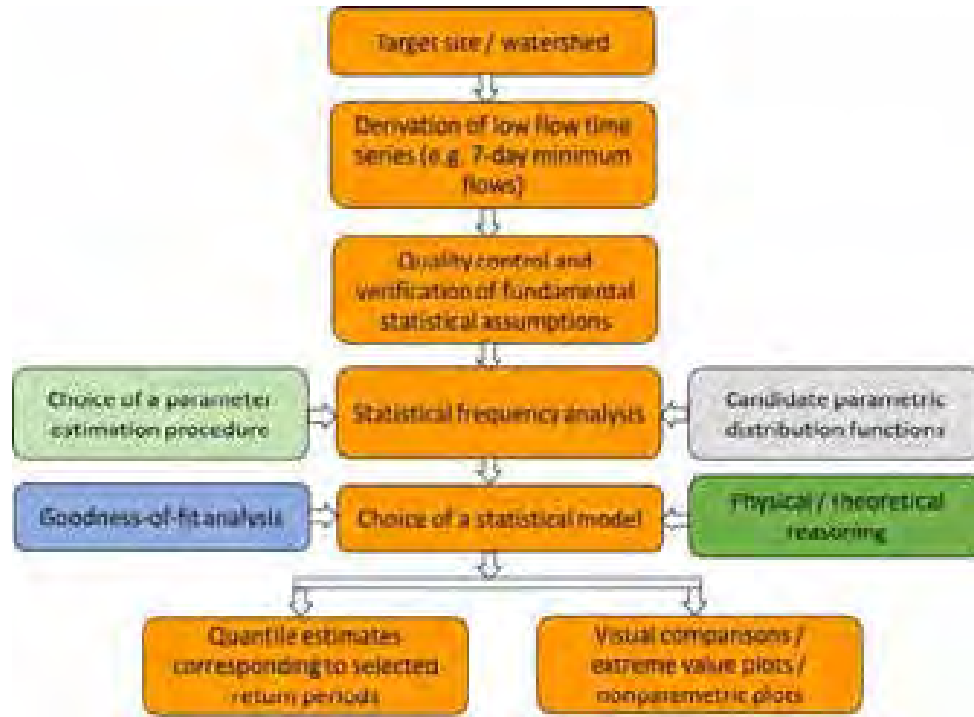
Figure 2.1: A process diagram showing various steps involved in at-site frequency analysis, starting from site selection to parameter estimation of distribution functions, choice of the model and outcomes of the entire process.
